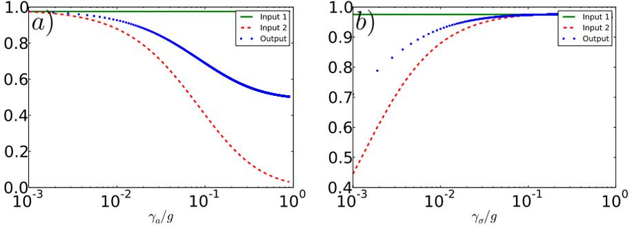
FIGURE 1. (Color online). Mean photon number of the input 1 (green, straight line), input 2 (red, dashed line) and output (blue, dotted line) states as a function of: a) the cavity's photon leakage rate  $\gamma_a$  and b) the excitonic decay rate  $\gamma_\sigma$  of the source 2. The output photon mean number is calculated uniquely for a 50:50 beam splitter, in which the photon mean number for both the output 1 and output 2 are equal.
