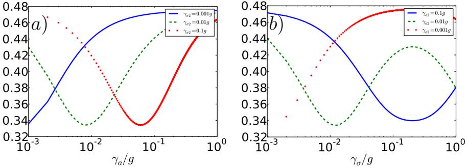
FIGURE 2. (Color online). Negativity of the output state as a function of: a)  $\gamma_{a2}$  for three different  $\gamma_{\sigma 2}$ , and b)  $\gamma_{\sigma 2}$  for three different  $\gamma_{a2}$ . In both cases, the negativity is maximum at the points for which  $\gamma_{a2} = \gamma_{a1}$  and  $\gamma_{\sigma 2} = \gamma_{\sigma 1}$ .
