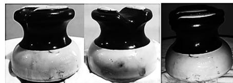
**Figure 5.** Pin ceramic insulator (ANSI 55-2) after 40 days of biological contamination with *Chlorella vulgaris*.
