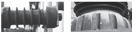
**Figure 2.** Insulators contaminated with algae. Rurópolis, Brazil.
