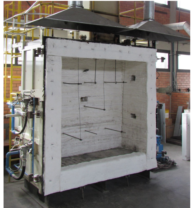
Figure 2. Vertical furnace used to determine the fire resistance of vertical sealing walls. Source: The authors.
