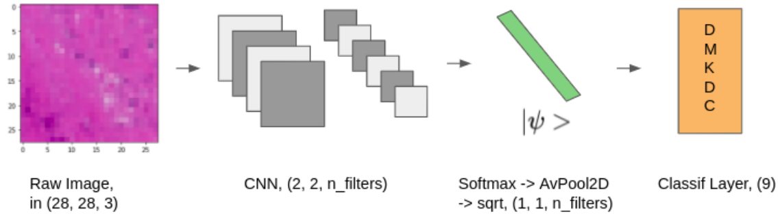
Figure 3.2.1: Method to combine CNNs with DMKDC. The images are represented as pure states to feed the DMKDC Classification layer
